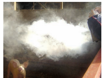
Check movement of air by using a smoke plume
